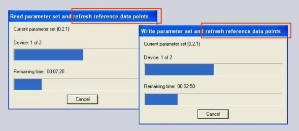
• After changing configuration parameters locally at the controller, refresh reference data points has still to be initialized manually (as it was up to now)
