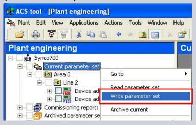
Select devices which shall be written and set Handling device, then go on with ok
