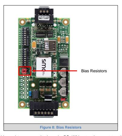
The ProtoNode bias resistors are used to keep the RS-485 bus to a known state, when there is no transmission on the line (bus is idling), to help prevent false bits of data from being detected. The bias resistors typically pull one line high and the other low - i.e. far away from the decision point of the logic.
