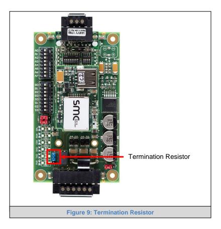
Termination resistors are also used to reduce noise. These pull the two lines of an idle bus together. However, they would override the effect of any bias resistors, if connected.
