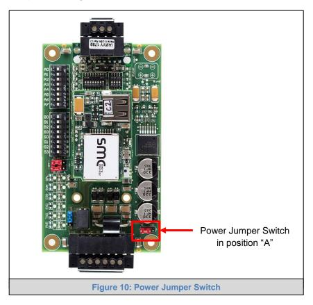
The ProtoNode Carrier Board power jumper is set to position A by default, but can be changed to position B for other power supply requirements.
