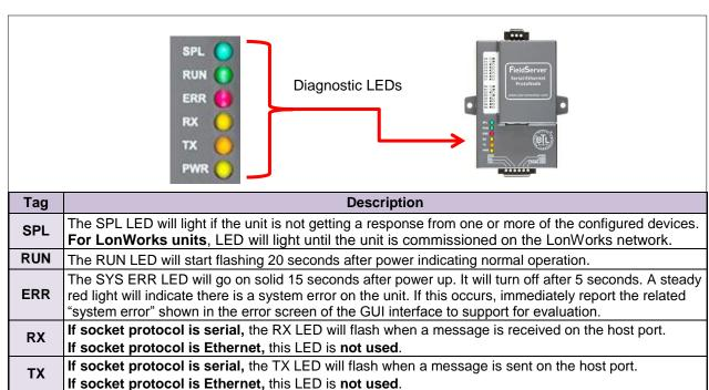
This is the power light and should show steady green at all times when the unit is powered.
