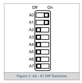
**NOTE:** When setting DIP Switches, please ensure that power to the board is OFF.
